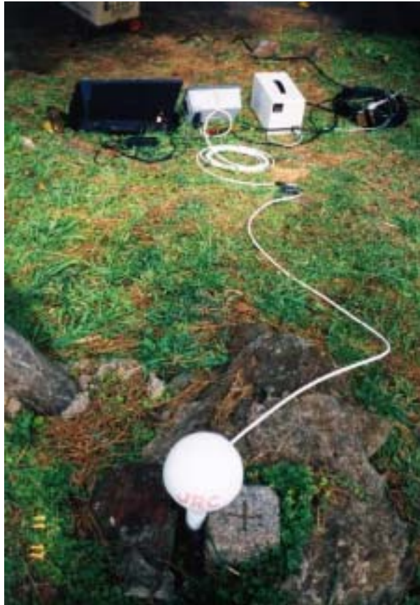
Fig. 3. Equipments for positioning at base point of Sarabong.
