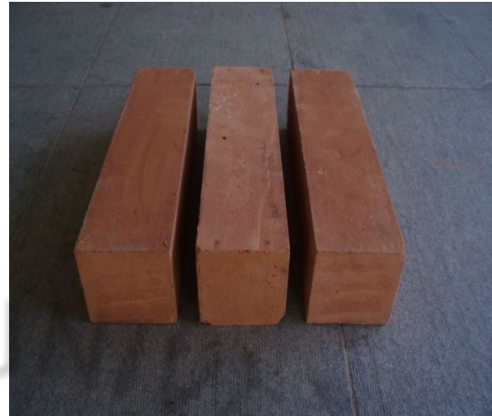
Fig. 4.5 The specimen for flexural strength with aggregate
