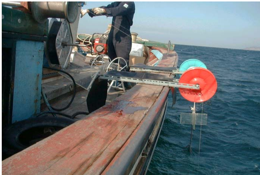
Fig. 17. The movement of resistance board in the sea test
