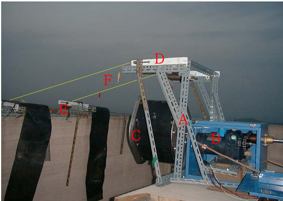
Fig. 13. Photograph of the rotary equipment for revolving a main line of continual squid hand line.
