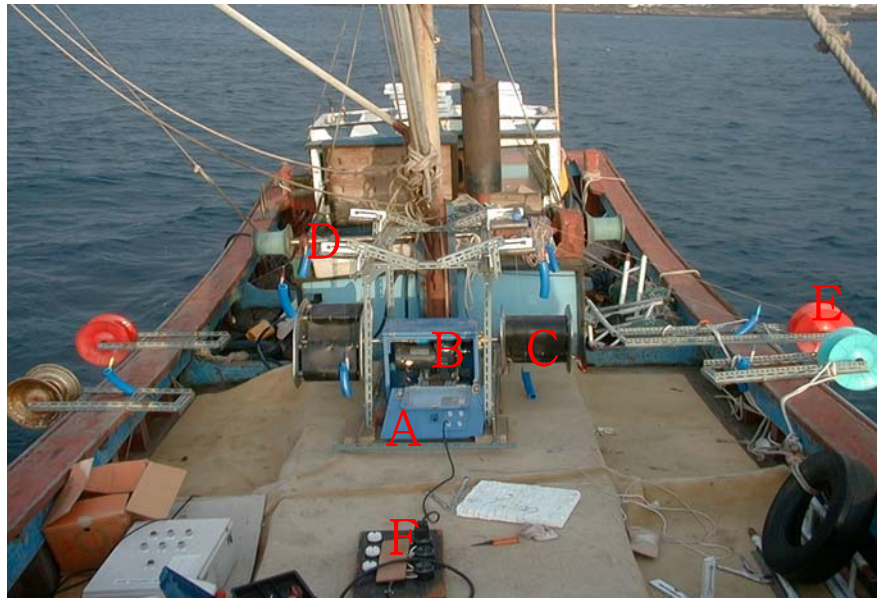
Fig. 16. Photograph of continual squid hand line in the sea test. (A) Inverter (B) Rotary equipment (C) Rotary drum (D) Inducement roller (E) Side roller (F) Hand dynamo
