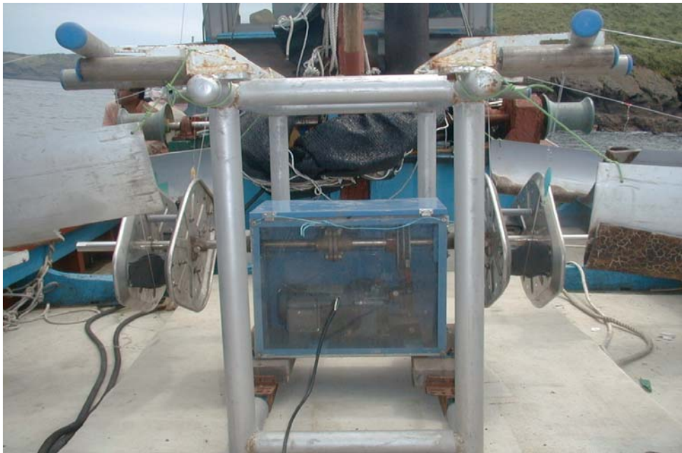
Fig. 6. The frame of continual squid hand line in the sea test.
