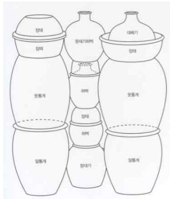
<Fig. 1> Laying Onggi in Gama(kiln) based on a line (Jeju National University Museum, 2011, p. 51)
