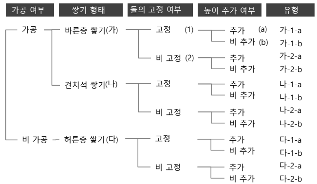
Fig. 6. Types of stone walls
