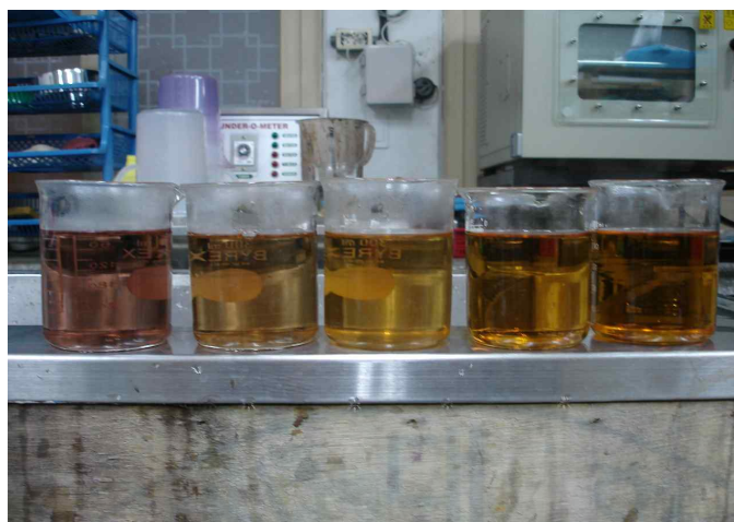
Fig. 5-14. Decoloration of samples in case of washing in hot water (from left sample 1, 2, 3, 4, 5).
