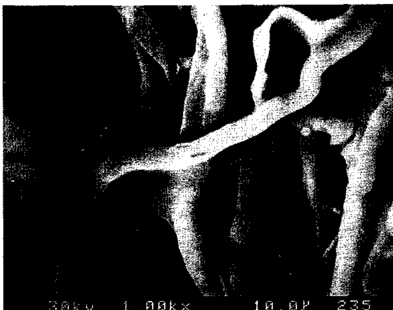
Plate 12. Scanning electron micrograph of cotton fabric dyed with persimmon juice ( \times 1000 )
