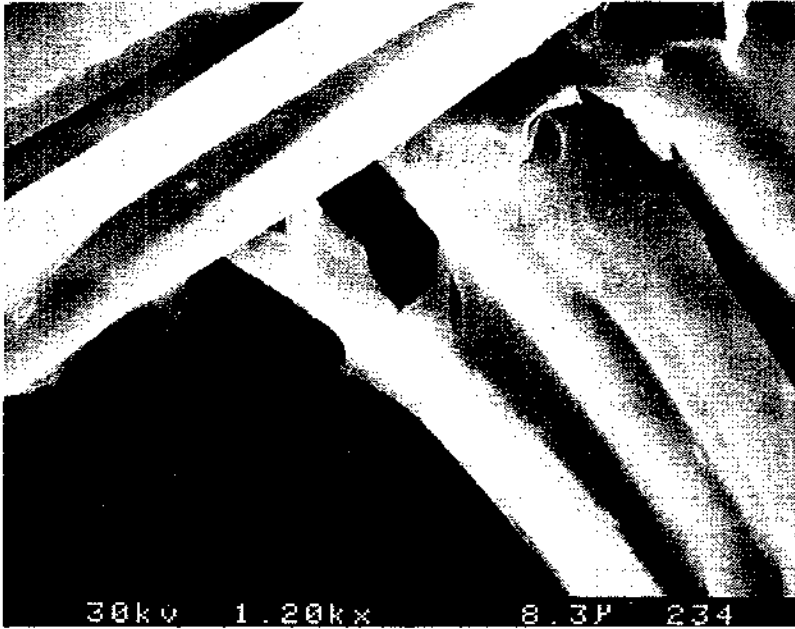
Plate 16. Scanning electron micrograph of silk fabric dyed with persimmon juice ( \times 1200 )
