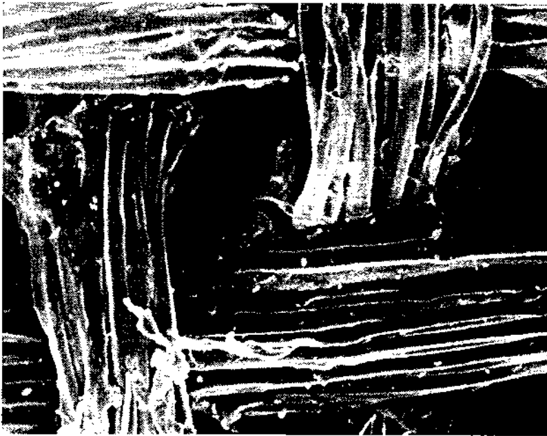
Plate 15. Scanning electron micrograph of silk fabric dyed with persimmon juice ( \times 300 )
