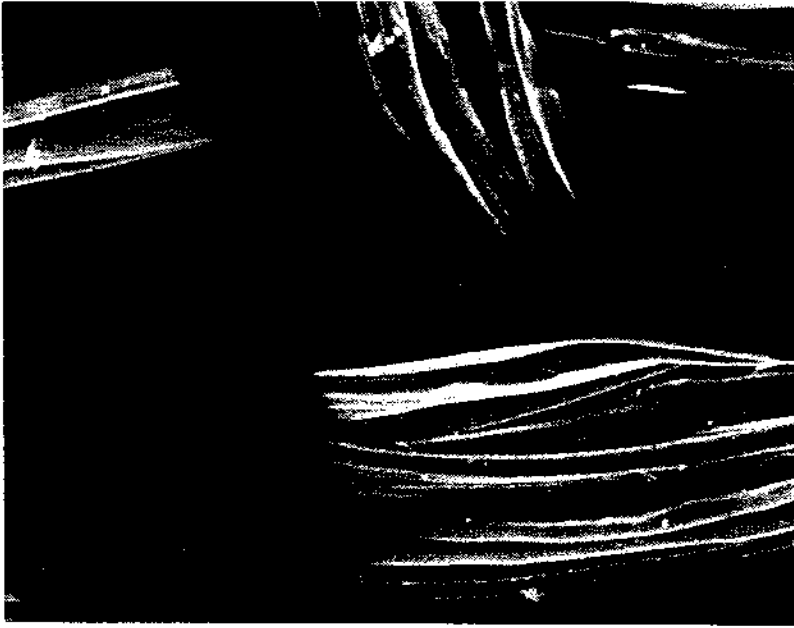
Plate 14. Scanning electron micrograph of natural silk fabric ( \times 300 )
