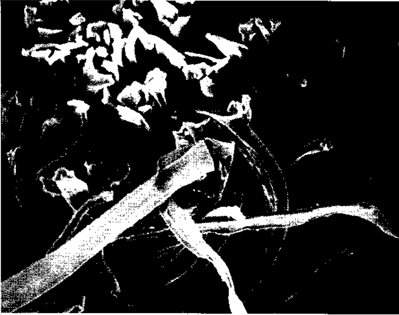
Plate 10. Scanning electron micrograph of natural cotton fabric ( \times 300 )
